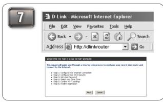
Open a web browser and enter http://192.168.0.1 or http://dlinkrouter. When the login window appears, select **Admin** as the username and leave the password box blank. Click **Log In** to continue the setup and follow the Setup Wizard. Please refer to the user manual for more detailed installation information and advanced features.
